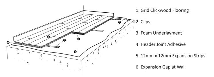
Grid Wood is engineered to perform with beauty. It is a portable system that boast a 3/8" sport foam shock pad and top layer of solid 7/8" thick Beech wood. Offered in a total system thickness of 1 ¼" thick with 8 colors including a Natural finish and 7 stain options. With Grid's innovative finishing technology, the factory applied finish is 3x stronger than any field applied finish.
